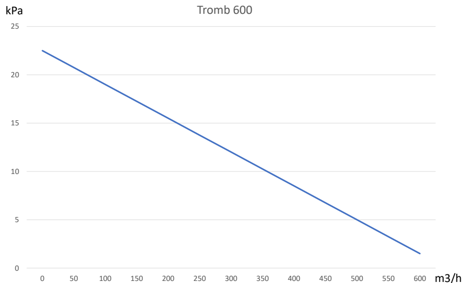
Pressure generation and air flow
